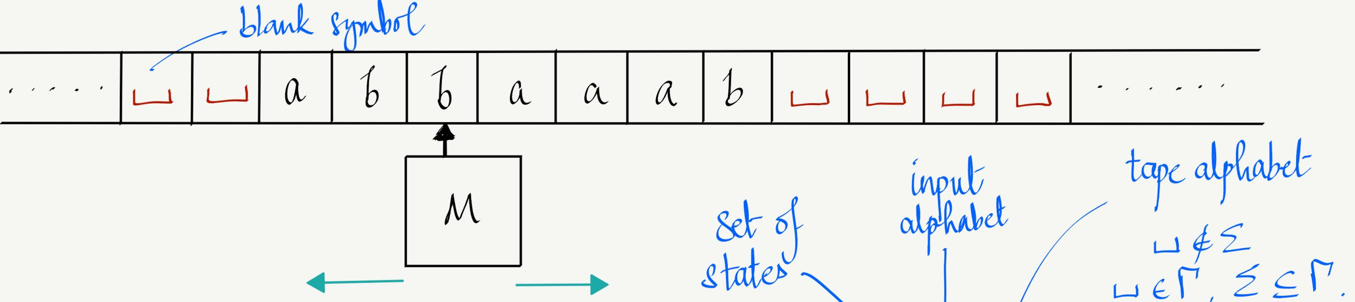
A deterministic\* Turing Machine:  $M = (Q, \Sigma, \Gamma, \delta, s, t, r)$
